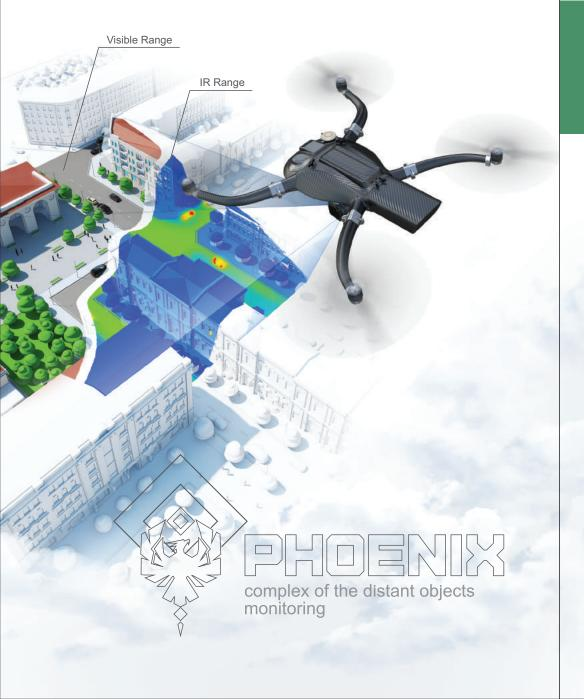
**Phoenix** complex uses unmanned aerial vehicle (UAV) and is designed for distant objects monitoring in the visible and infrared ranges. It is applicable as a separate product and as a part of other complex security systems.
