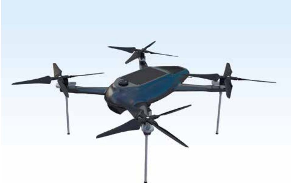
Carbon body and propeller blades
